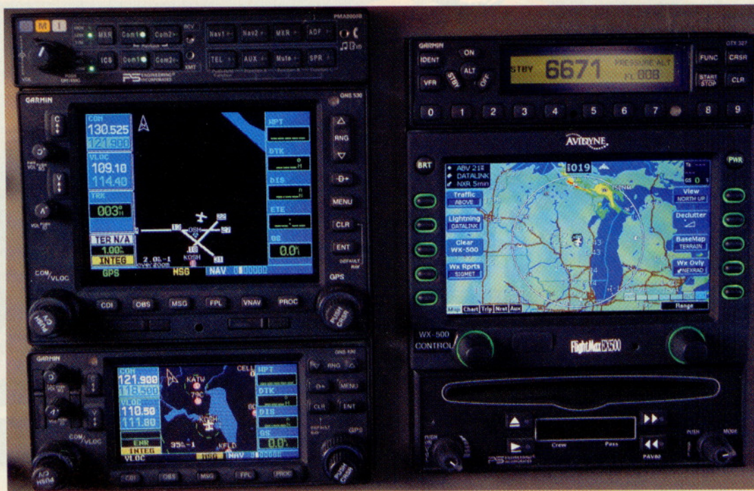
The core of the Win a Six's communications and navigation avionics. Top to bottom and left to right, is a PS Engineering PMA8000 audio panel; a Garmin GNS 530 and 430 GPS/nav/com package; a Garmin GTX 327 transponder; an Avidyne EX500 multifunction display; and a PS Engineering PAV80 AM/FM radio/CD and DVD player. Note how the Heads Up Technologies satellite receiver plots Nexrad returns on the EX500.
